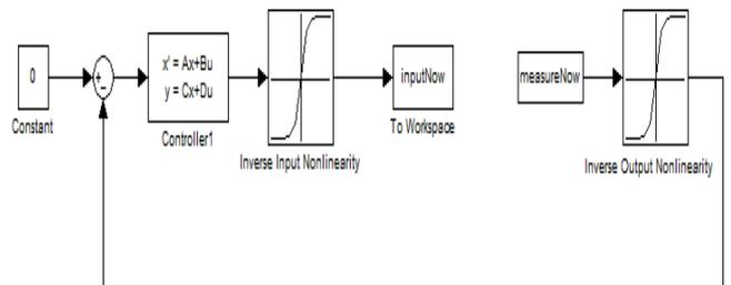
Fig. 7. SIMULINK block diagram for the controller's operation during closed-loop simulations.
