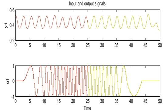
Fig. 2. The Chirp signal input ( $u_1$ ) and the resulting measured output ( $y_1$ ).
