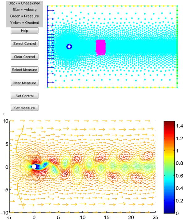
Fig. 1. Selected actuation and measurement points of the Navier2d program (upper) and the velocity field resulting from running the CFD simulation for about 250 seconds (upper).
