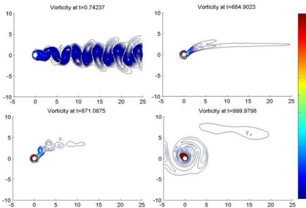
Fig. 8. Vorticity values of the flow field at indicated times.
