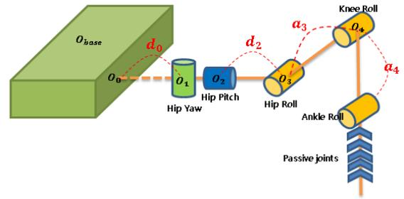
Fig. 11. Kinematic modeling of the leg.
