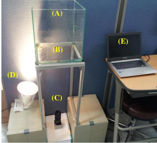
Fig. 3. A motion capture system - (A): A transparent water tank, (B) : Diving beetles, (C): A high-speed camera, (D): A lamp, (E) : A laptop computer.
