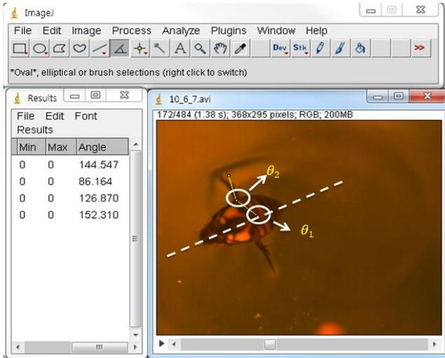
Fig. 4. Image processing by Image J to measure the joint angles on the leg of the diving beetle.
