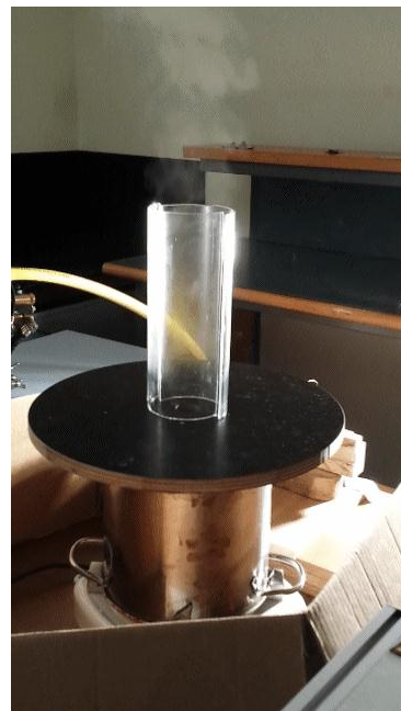
Fig. 2(a). Experimental set-up for swirl visualization.
