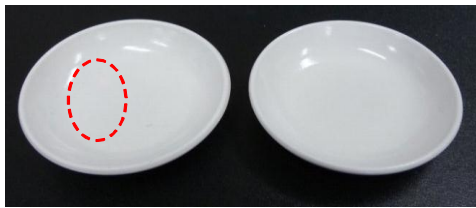
Fig. 7. Left: With glass phosphor. The material is added in the area of dashed line. Right: without glass phosphor.
