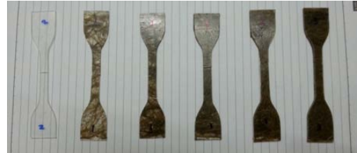
Fig. 3. Tensile specimens with varying M_f (from left: 0%, 4.3%, 7.8%, 10.4%, 12% and 15.2%).
