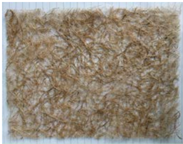
Fig. 2. EFB palm fibre mat prepared through hand lay-up.
