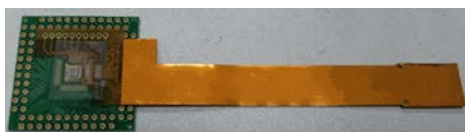
Fig. 2. A flexible capacitive tactile sensor array with a readout chip.
