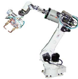
Fig. 5. Spot welding machine gun attached with robot.
