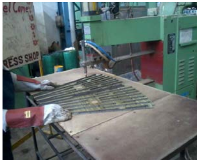
Fig. 4(b). Operator performing the spot welding.
