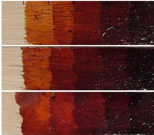
Fig. 10. Sample coated with clear lacquer and glass phosphor powder. (Top: 10%, Center: 5%, Bottom: 1%).
