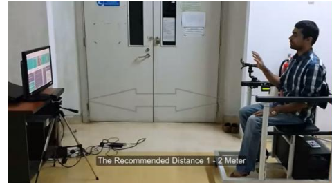
Fig. 4. Setup of motility with kinect system.
