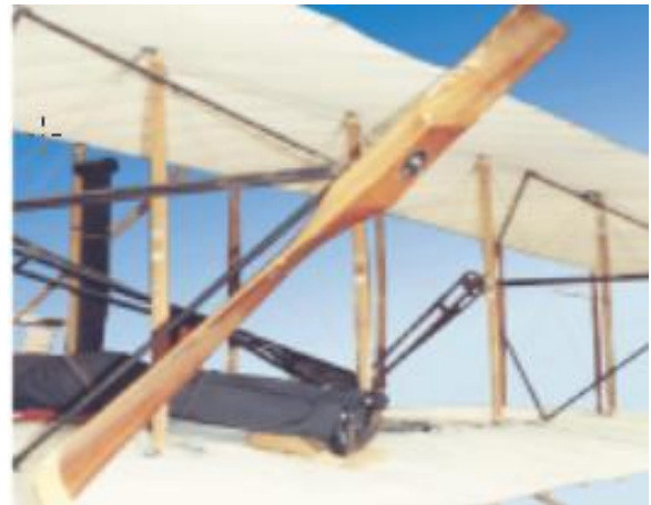
Fig. 2. Wright Brothers fixed pitch twin bladed propeller.
