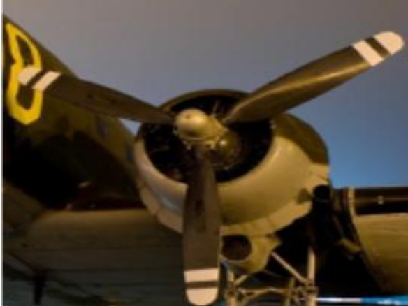
Fig. 4. Twin pitch propeller on a DC-3 aircraft.
