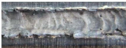
Fig. 1. Surface morphology of \text{CeO}_2 powder cladding coating.
