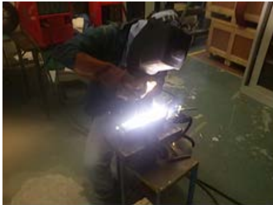
Fig. 3. Shielded metal arc welding.
