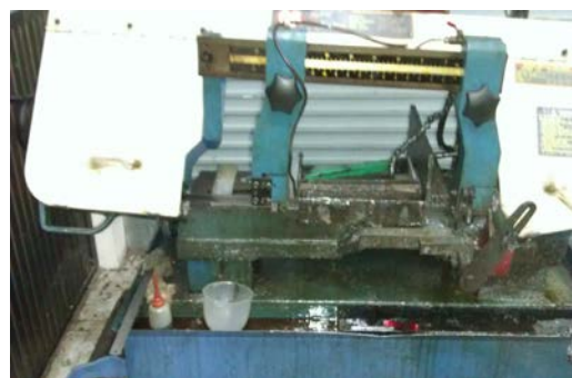
Fig. 5. Cutting with square-band saw.
