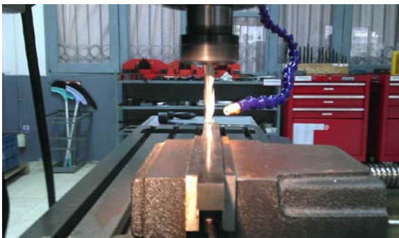
Fig. 7. Face milling the specimens.
