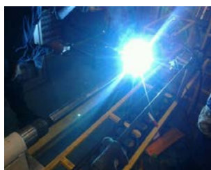
Fig. 15. Propeller shaft hardfacing.
