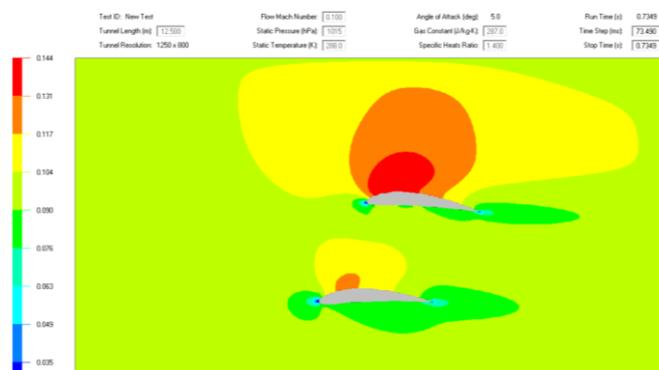
Fig. 3. Twin-wing and positive stagger with lower AoA  $0^\circ$ .
