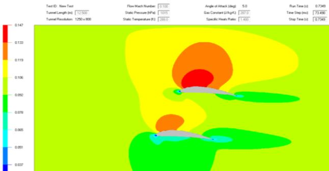
Fig. 5. Twin-wing and positive stagger with lower AoA  $5^\circ$ .
