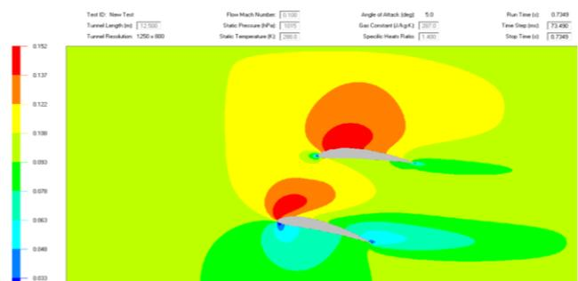
Fig. 8. Twin-wing and positive stagger with lower AoA  $15^\circ$ .
