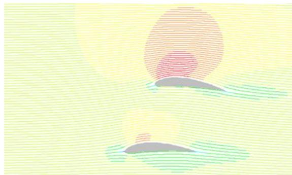
Fig. 4. Laminar flow and downwash.
