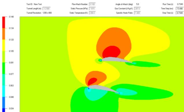
Fig. 6. Twin-wing and positive stagger with lower AoA  $10^\circ$ .
