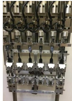
Fig. 1. Fatigue setup-up with samples at fully-relaxing conditions.
