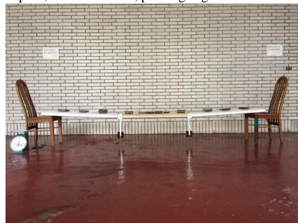
Fig. 3. Wing is under 42 (kg) loading test.
