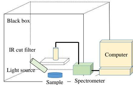
Fig. 7. Light emission spectrum observation system.
