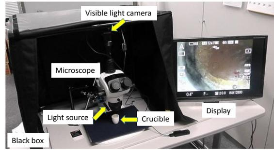
Fig. 6. Visible light emission observation system.
