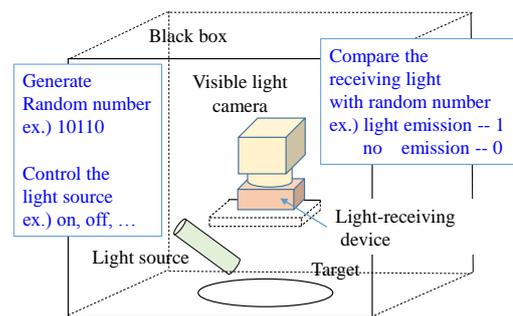
Fig. 22. Detecting fake product by using light modulation.
