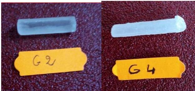
Fig. 4. Effect of Li<sub>2</sub>O addition on the structure and opacity of studied glass system (B<sub>2</sub>O<sub>3</sub>-ZnO).
