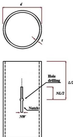
Fig. 2. Geometrical parameters of specimens.
