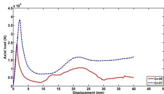
Fig. 11. Comparison between load-displacement diagrams of specimens Cn-08 and Cn-01 with  $t=0.75$  and 1mm.
