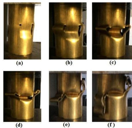
Fig. 8. Inward and outward folding of specimen Cn-07.
