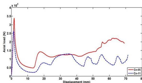
Fig. 12. Comparison between load-displacement diagrams of specimens Cn-05 and Cn-11 with tube outer diameters of  $d=35$  and 50 mm.
