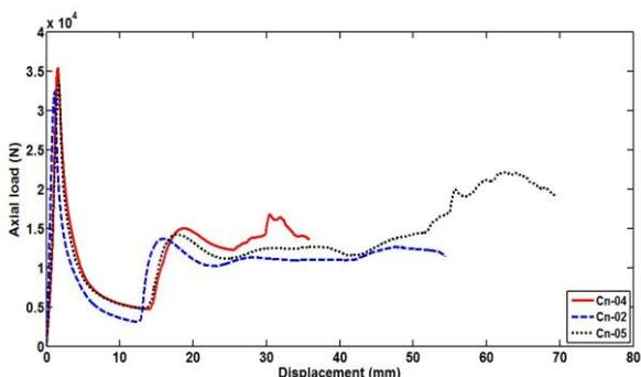
Fig. 10. Comparison between load-displacement diagrams of specimens Cn-04, Cn-02 and Cn-05 with  $L=50, 70$  and 100 mm.
