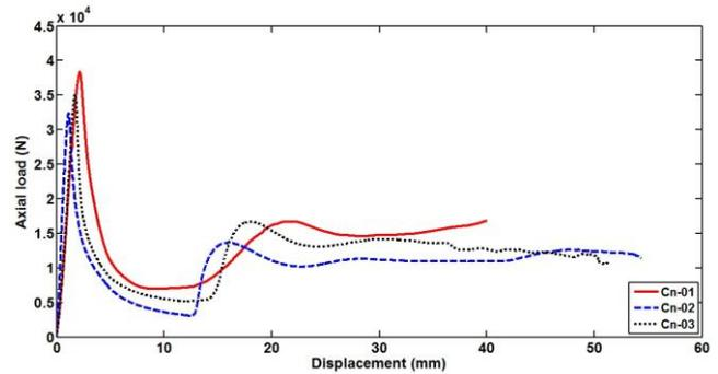
Fig. 6. Comparison between load-displacement diagrams of specimens Cn-01, Cn-02 and Cn-03 with  $n=4, 6$  and  $8$ .
