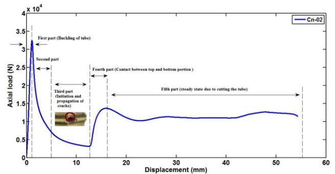
Fig. 5. Different steps of load-displacement diagram of specimen Cn-06.
