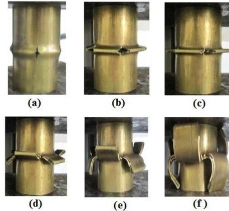
Fig. 4. Specimen Cn-02 during axial splitting process.
