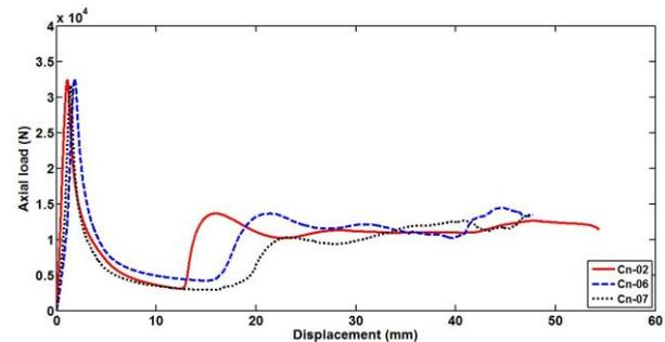
Fig. 7. Comparison between load-displacement diagrams of specimens Cn-02, Cn-06 and Cn-07 with  $NL=10, 14$ , and  $18$  mm.
