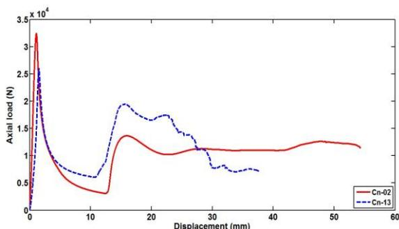
Fig. 9. Comparison between load-displacement diagrams of specimens Cn-02 and Cn-13 with  $NW=1$  and 3 mm.
