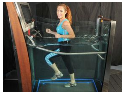
Fig. 4. The underwater treadmill using buoyancy vests in pools to help injured athletes keep their fitness levels up [12].
