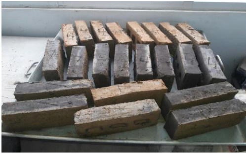
Fig. 3. Modified bricks after molding.
