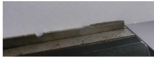
Fig. 12. Fracture of MT specimen.
