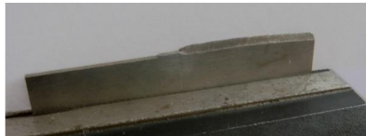
Fig. 13. Fracture of CT specimen.
