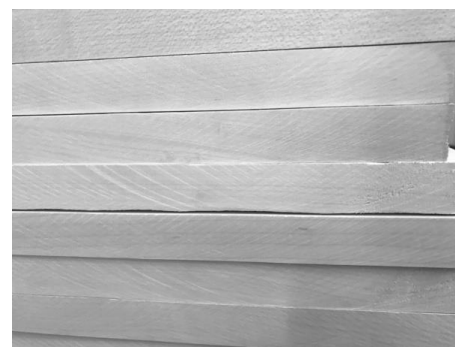
Fig. 2. Drifting in the sawing process creates obvious saw marks.
