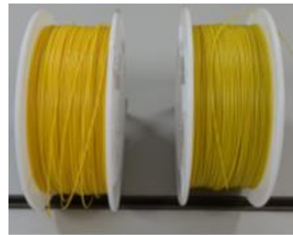
Fig. 4. Filaments made of these ABS resins. The filament on the right contains dye, one on the left is pure one.
