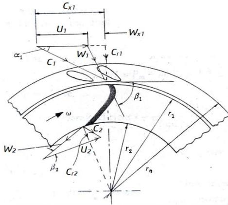
Fig. 2. Velocity triangles for a Francis turbine.
