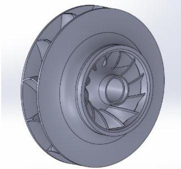
Fig. 5.1. The 662mm turbine runner model.
