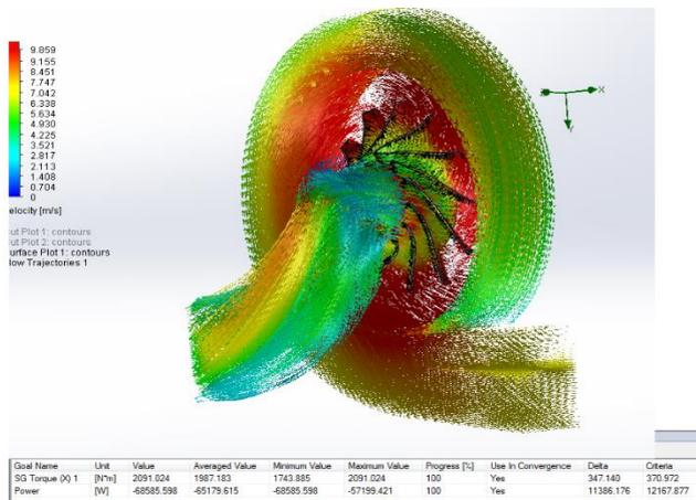
Fig. 5.2. Velocity profile and flow trajectories of the PAT using solid works flow simulation.
