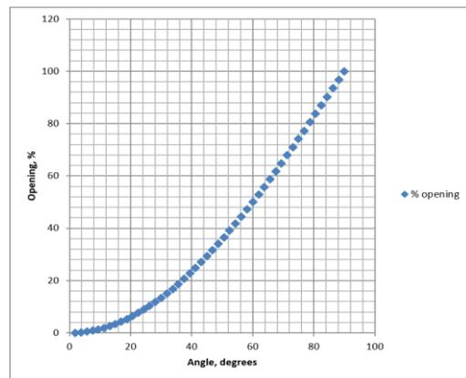
Fig. 4.2. Percentage opening angle of turn of butterfly valve.
