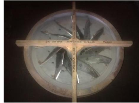
Fig. 7. Pattern for the inner part of the runner.
