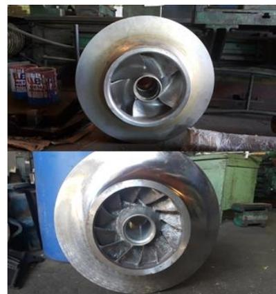
Fig. 9. Comparison between original impeller and the turbine runner.
