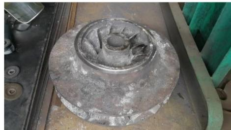
Fig. 8.1. Side view of the casted runner.
