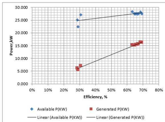
Fig. 11. Relationship between available and generated power by PAT.
