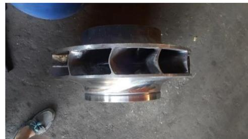
Fig. 8.2. The runner after machining.
