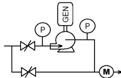
Fig. 4.1. Schematic diagram of the bypass pipeline.
