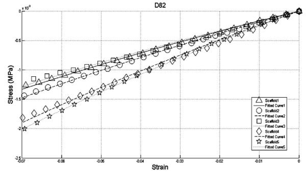
Fig. 1. Curve Fitting of Gelatin/CMC (D82) Scaffolds.
