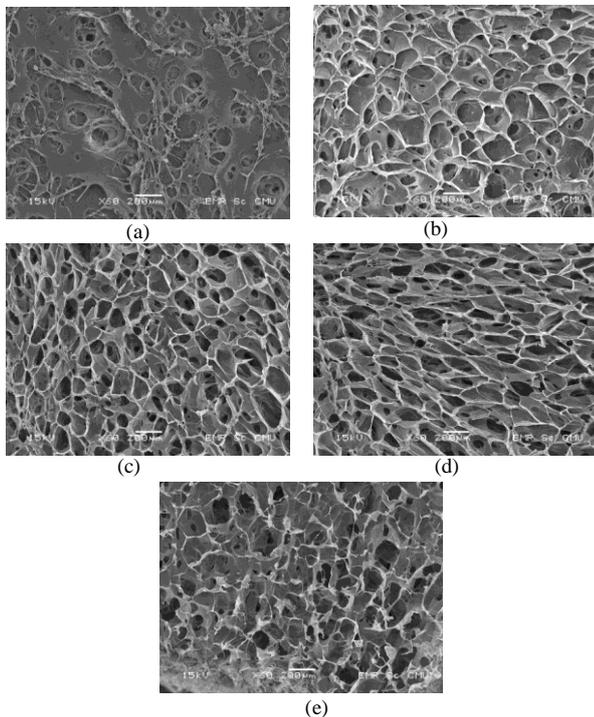
Fig. 3. SEM images of dehydrothermal treatment scaffolds (a) D100 (b) D91 (c) D82 (d) D73 and (e) D64.
