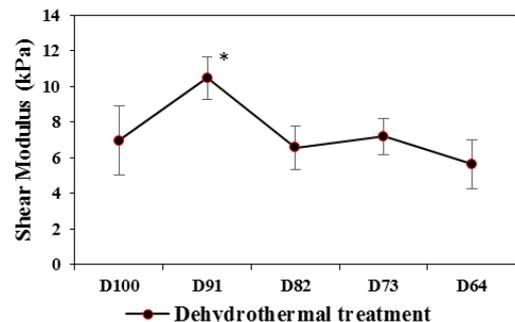
Fig. 2. Summary of Initial Shear Modulus of gelatin/CMC Scaffolds ( $n=5$ ) (\* significant different  $p < 0.05$  relative to D100).
