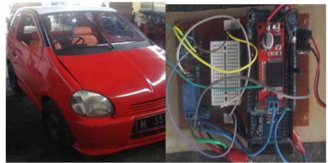
Fig. 11. The application of automatic wiper system, (a) wiper application on electric car, and (b) electronic controller hardware chain.
