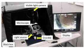
Fig. 6. Visible light emission observation system.
