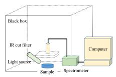
Fig. 7. Light emission spectrum observation system.
