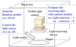
Fig. 22. Detecting fake product by using light modulation.
